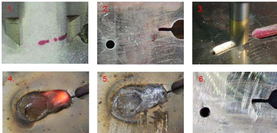
Figure 7: Preparation of the CT-specimen “welding 02” for the second test phase; 1. dye penetrant inspection; 2. drilling of the crack tip; 3. removal of the damaged metal; 4. repair welding; 5. removal of slag; 6. grind of welding seam elevation
