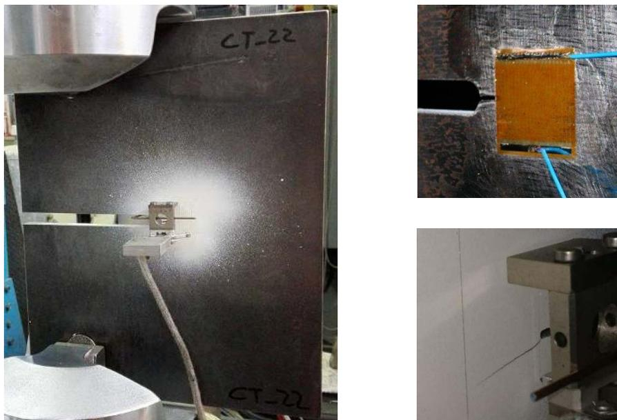
Figure 8: Test setup; left: CT-specimen in the testing machine; upper right: Detail of the RDS propagation gauges; lower right: Extensometer and white painted area for visual crack control
