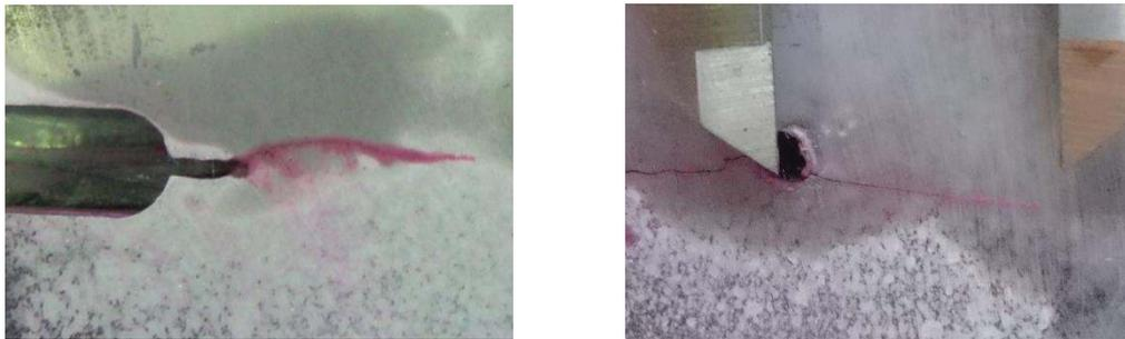
Figure 6: Dye penetrant inspection; left: After the first test phase (specimen “welding 01”);
